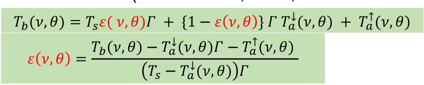
$T_h(\nu, \theta)$ : brightness temp.  $\nu$ : frequency,  $\theta$ : zenith angle  $T_s$ : land surface temp. (LST)  $T_a^{\downarrow}$ : downwelling  $T_b$ upwelling  $T_{h}$  $\Gamma$ : transmissivity
