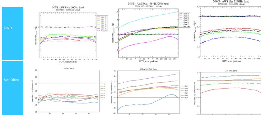
**Figure 3.** Cross scan O-B difference for each of the main bands in the AWS radiometer. The *top row* are from DWD monitoring, the *bottom row* from Met Office monitoring
