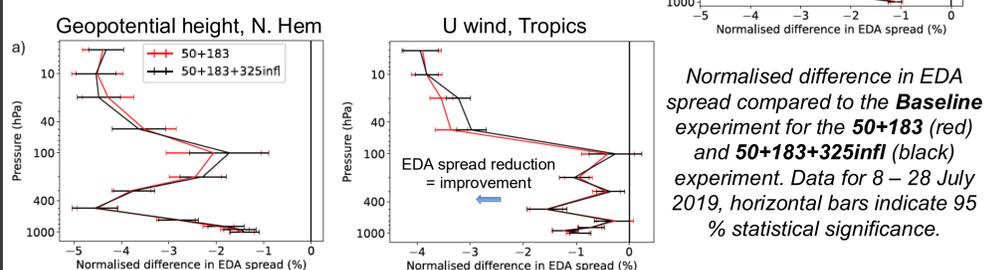
Using the three channel sets together, EPS-Sterna has a very clear positive impact, though the contribution of the 325 GHz channels is comparatively small. Further enhancements of the assimilation approach may improve the impact of the 325 GHz channels.
