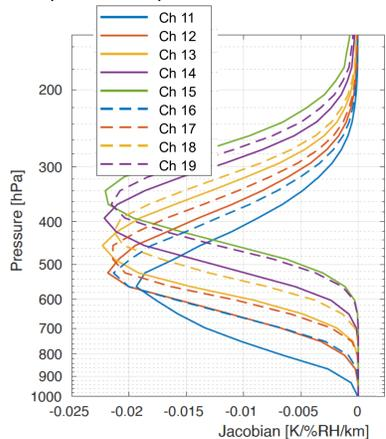
325 GHz channels (16-19) peak at similar altitudes as corresponding 183 GHz channels (11-14).
