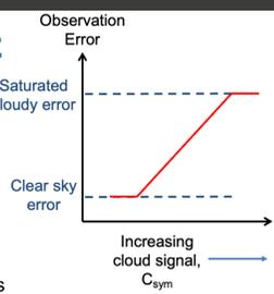
Clear-sky errors are calculated from the NEDT using empirical formulae as for the 183 GHz channels. For the cloudy errors, values are taken from corresponding 183 GHz channels from heritage sensors, scaled by the ratio of standard deviations of cloud-affected background departures for the 325 and 183 GHz channels.
