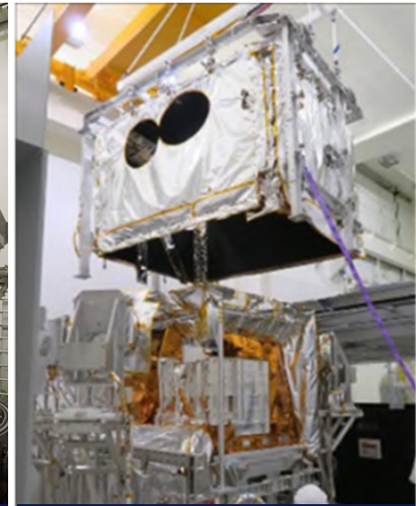
THERMAL TENT INSTALLATION (COURTESY OF AIRBUS)
