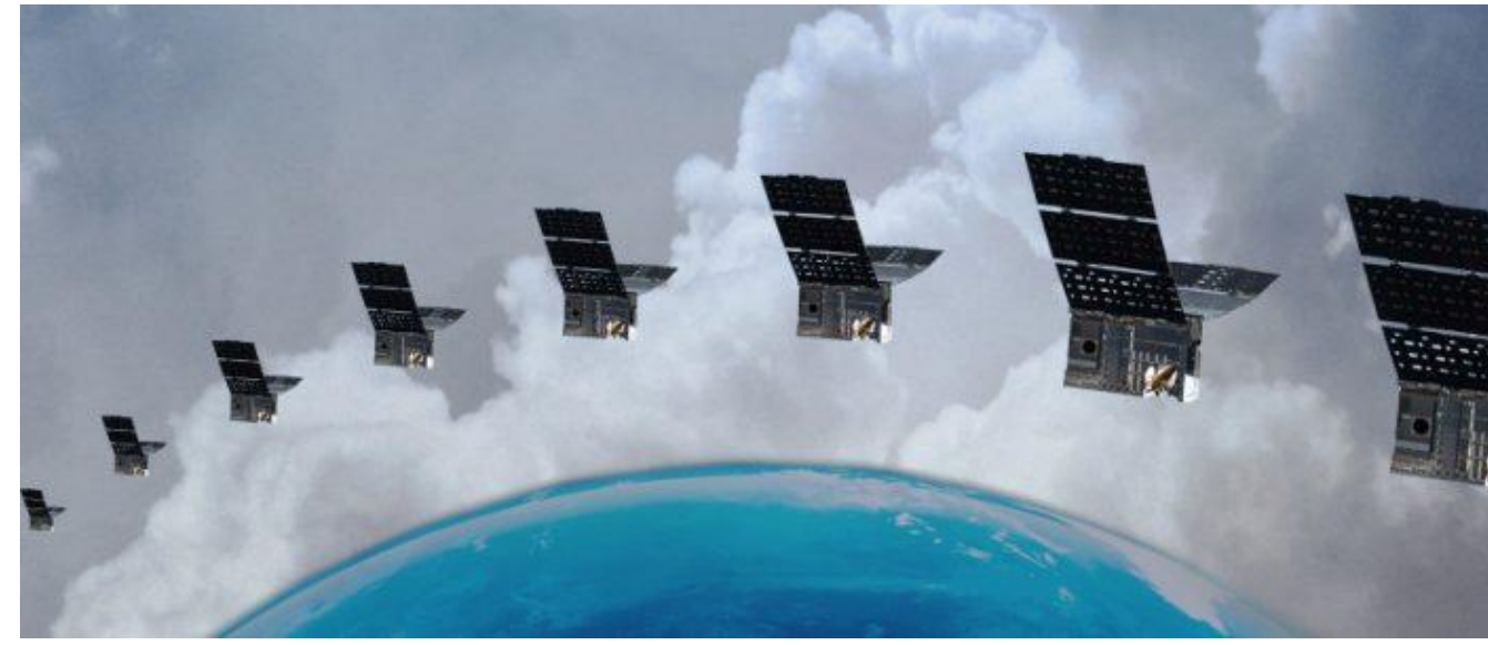
8-satellite constellation concept of TEMPEST providing high temporal resolution observations ( https://tempest.colostate.edu/ )
