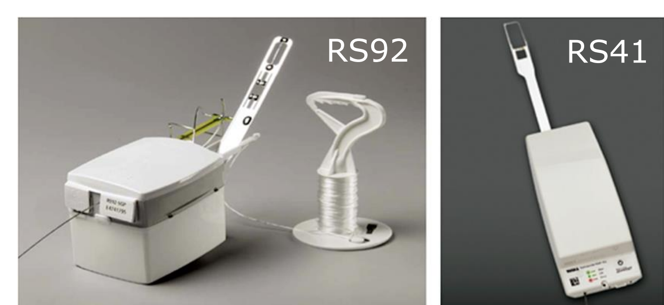
Figure 2. Vaisala RS41 radiosonde has been replacing the Vaisala RS92, becoming the major sonde type across the GRUAN and Conventional radiosonde networks. (courtesy of https://www.vaisala.com ).
