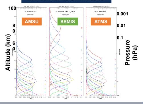
Of the current Microwave Sounders only the **SSMIS Upper Atmospheric Sounder (UAS)** covers the mesosphere ~50-85km and lower thermosphere.
