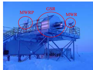
Figure 1. The experimental set-up on the ARM GWT deck during the WVIOP2004. The microwave radiometers (ARM MWR and MWRP, NOAA/ETL GSR) are circled in red.
