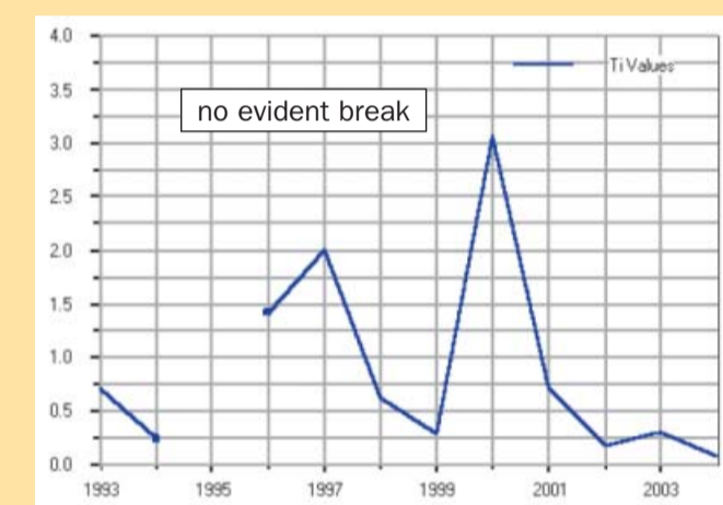
SNHT values for 'satellite' total ozone series for Belsk vs ground measurements for April
