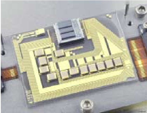
FPA module achieved 100% operability in all channels
