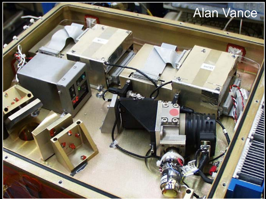
ARIES with starboard side removed showing electronics modules (top), detector/cooler unit (bottom right), heater controller (mid left) and folding/focusing optics (bottom left).
