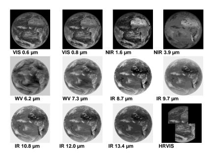
Figure 5: MSG capabilities: Example images from 12 SEVIRI Channels.
