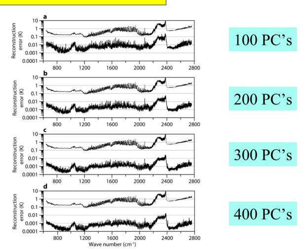
In the PC based RTTOV, the simulated PC scores are computed using a linear regression scheme where the independent variables (predictors) are a selected number of polychromatic top of the atmosphere radiances computed using the standard RTTOV fast transmittance model.
