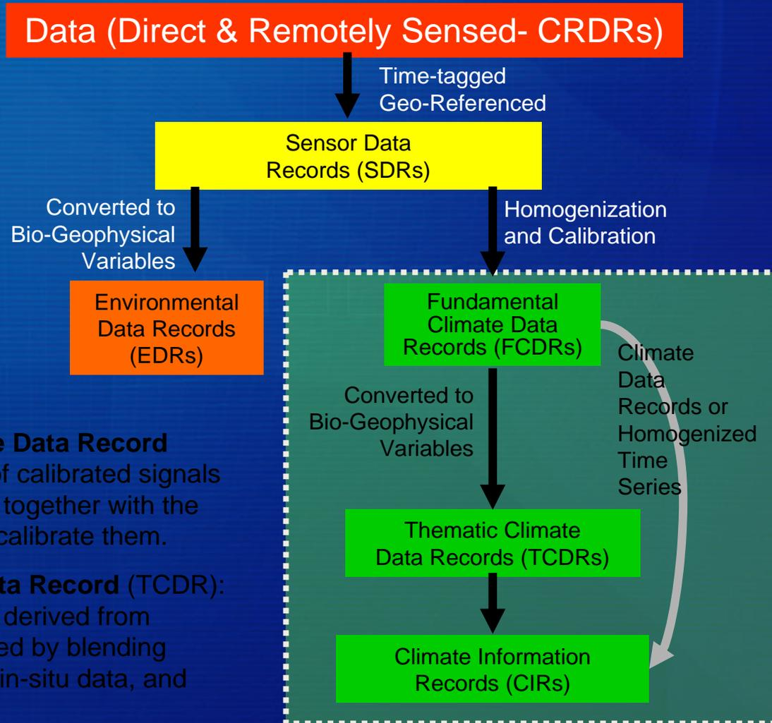
**Fundamental Climate Data Record (FCDR):** Time series of calibrated signals for a family of sensors together with the ancillary data used to calibrate them.
