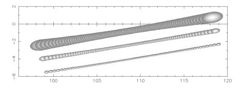
Figure 1. Nominal 50% power ATMS fovs. The gray scale indicates the relative power, with the center being 100% power and the edge being 50% power. Shown are the three resolutions of the ATMS. The coordinates are latitude and longitude.
