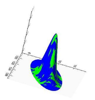
Figure 4. ATMS 5.2° fov at the 99% power level, with DEM warped over the relative antenna power.
