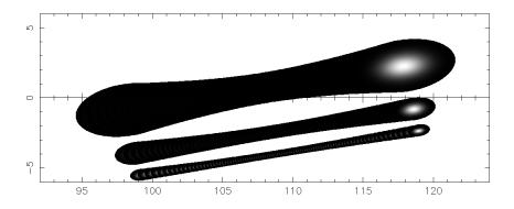
Figure 2. ATMS fovs at 99% power. The gray scale indicates the relative power, with the center being 100% power and the edge being 1% power. Shown are the three resolutions of the ATMS. The coordinates are latitude and longitude.
