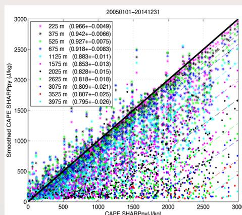
CAPE computed from vertically smoothed sonde temperature and moisture profiles compared to CAPE computed from full resolution vertical sounding at 75 meter resolution. The legend indicates the boxcar smoother full width in meters and the linear regression slope fit.
