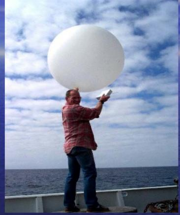
National science vessels (like NOAA Ronald H Brown) often include automated (ASAP) radiosonde, in-situ measurement (cloud, radiometric, SST) capability ... optimal platform for REFRENCE network!
