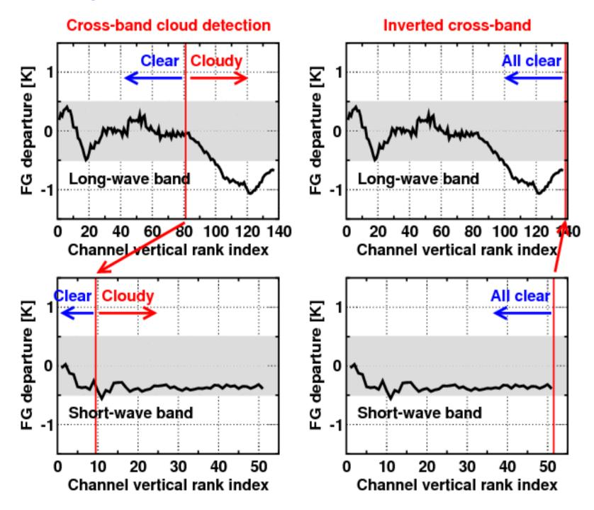
The operational setup of the Integrated Forecast System (IFS) at ECMWF applies a cross-band option in cloud detection. This means that channel-specific cloud flags for the whole of infrared spectrum are assigned on the basis of FGD data on long-wave (LW) channels only.
