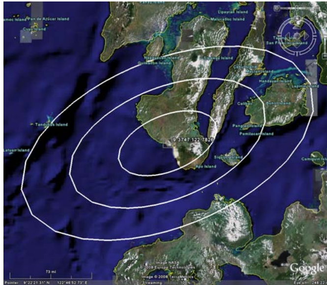
Figure 3. Nominal 50% power AMSU fov (inner) with 95% and 99% power fov over the Philippines.
