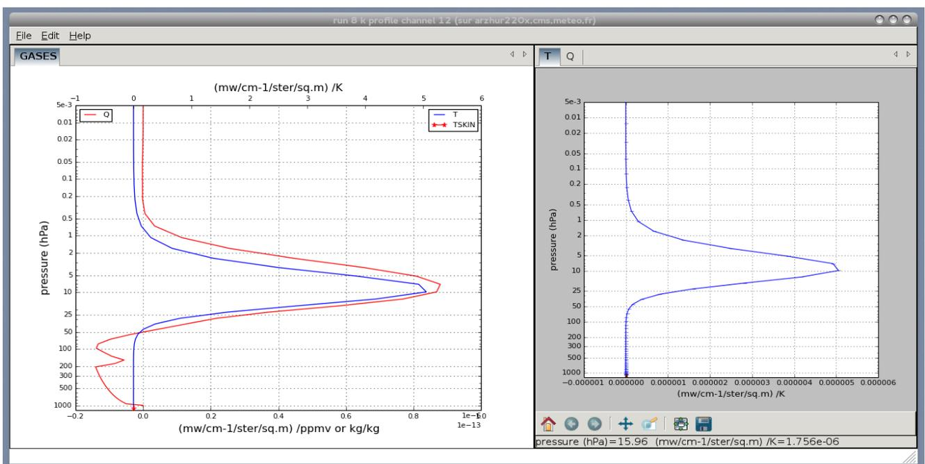
Figure 10 K: profile window displaying a Jacobian for METOP-1/AMSUA channel 12.
