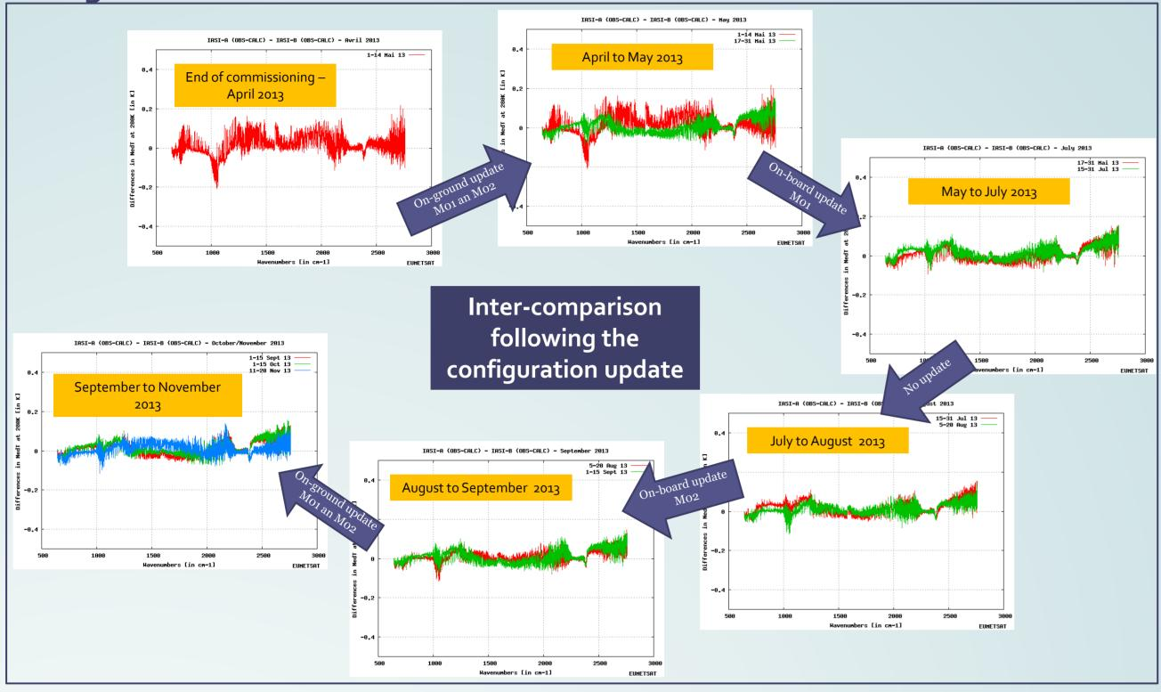
The difference in NedT at 28oK remains between ± 10<sup>-1</sup> K (the specification for Obs-Cal is 0.1K at 28oK), which shows a good radiometric consistency between the two IASI. One can follow the configuration evolution quite accurately, giving a status of the two IASI inter-calibration. The last configuration update gives the best fit between the two instruments. Note that this monitoring is done for 15 days per month, taking into account any configuration change.
