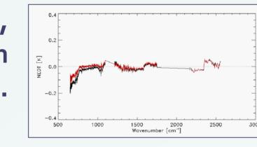
The radiance comparison of IASI and HIRS on-board Metop is performed on all pixels with a distance smaller than 3 km between IASI and HIRS. All sky conditions are included (clear, cloudy, day and night). The radiance differences IASI - HIRS are given in NedT at 28oK. On the figures below are shown the average and standard deviation for all HIRS channels in clear situations for day and night conditions, Metop-A and the left and Metop-B on the right. The comparison between HIRS and IASI on
