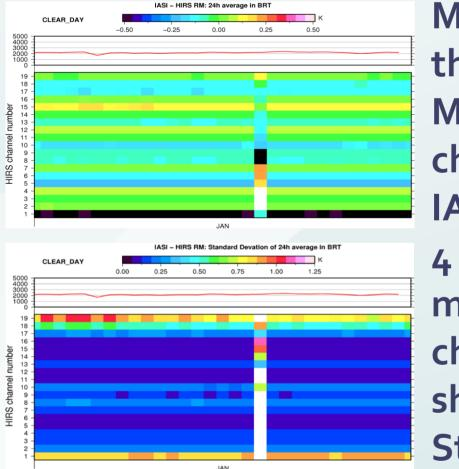
Metop-B are a bit different than the one done on Metop-A. Some HIRS-B channels are colder than IASI-B-like for the channel 4 and some others are much warmer like the channel 15 and 16, as shown on the figures (Avg, Std) on the left and right.
