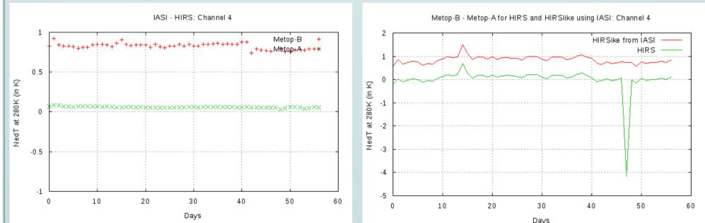
the difference observed is coming from the HIRS instrument Spectral Response function used.
