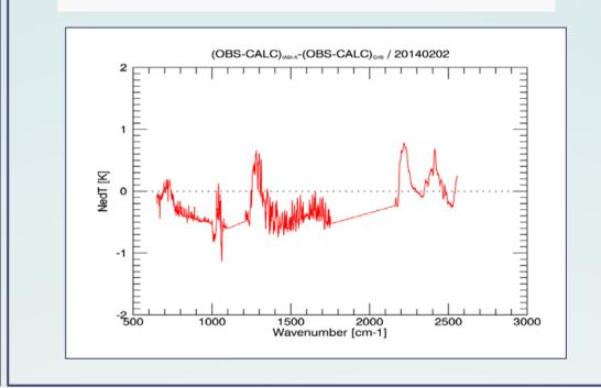
The (Obs-Calc) differences are not as good as the ones from SNOs. More cloud filtering needs to be done. We see that, in general, CrIS is slightly warmer than IASI in band 1, with some remaining non-linearity. A new comparison, shown on the figure below, has been done with a new version of the products, and one can notice an improvement (red curve).
