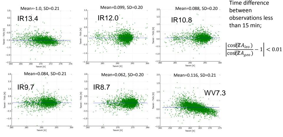
Statistical comparison of outgoing radiation measurements by 3 instruments: IRFS-2 and IASI-A, -B : Difference between SD of radiances: IRFS-2 minus IASI
