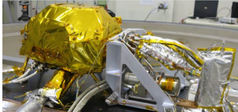
Equipped cryostat under thermal vacuum testing
