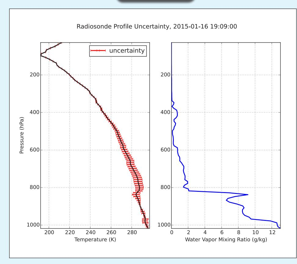
Temperature and water vapor profiles for a clear sky scene, obtained from a radiosonde (above). Radiative transfer calculation with LBLRTM and obs-calc comparison with the M-AERI observed radiance (above right). Radiance Jacobians from the OSS radiative transfer model were used to calculate the uncertainty in the atmospheric profile (error bars, above).
