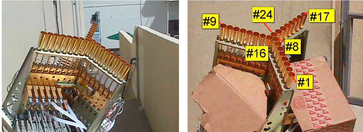
a) Initial configuration b) Final configuration Fig. 6: GeoSTAR prototype outdoors to observe the sun’s transit
