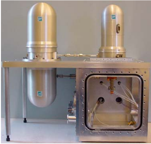
Figure 4. Ball Aerospace & Technologies Model SB235 Cryocooler
