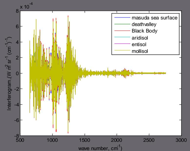
Exemplifying the concept of emissivity as a low frequency component through spectra with different emissivity, but same atmospheric state vector. The Difference with the Black Body spectrum show that the emissivity is seen at low frequency but not at high frequency
