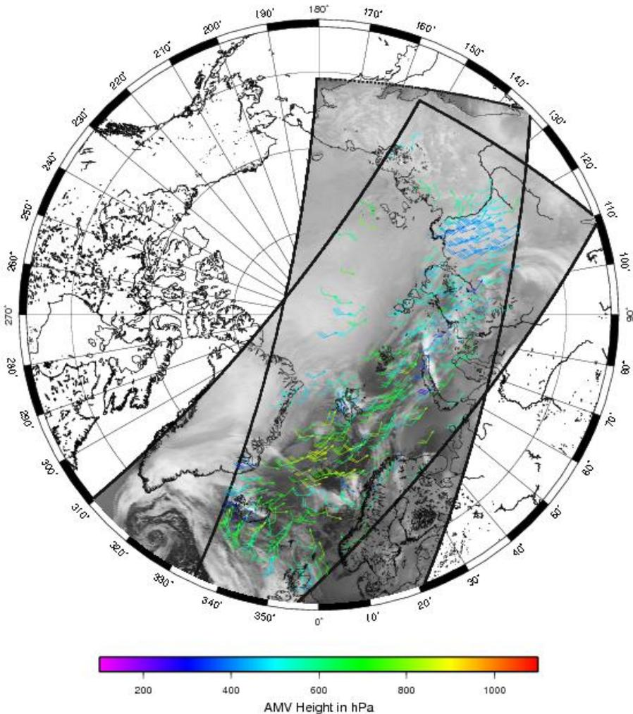
Mapping of AVHRR/3 data over the poles onto a common projection
