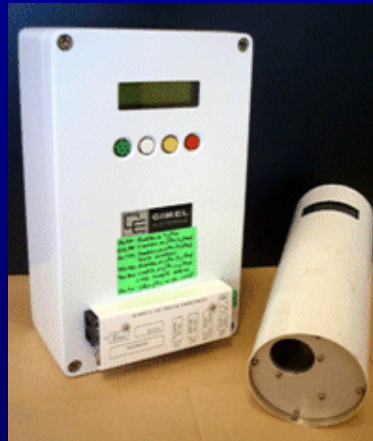
CIMEL CE 312-2 thermal radiometer (5 channels matching ASTER bands and 1 broad channel 8-13 \mu\text{m} )
