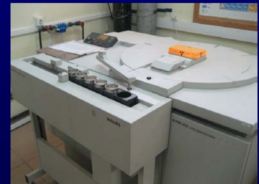
X-Ray Spectrometer (PW-240) to determine chemical composition
