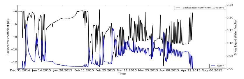
Comparison between the simulated backscatter coefficient and the snow liquid water fraction of the snowpack (beginning of 2015/2016 season)
