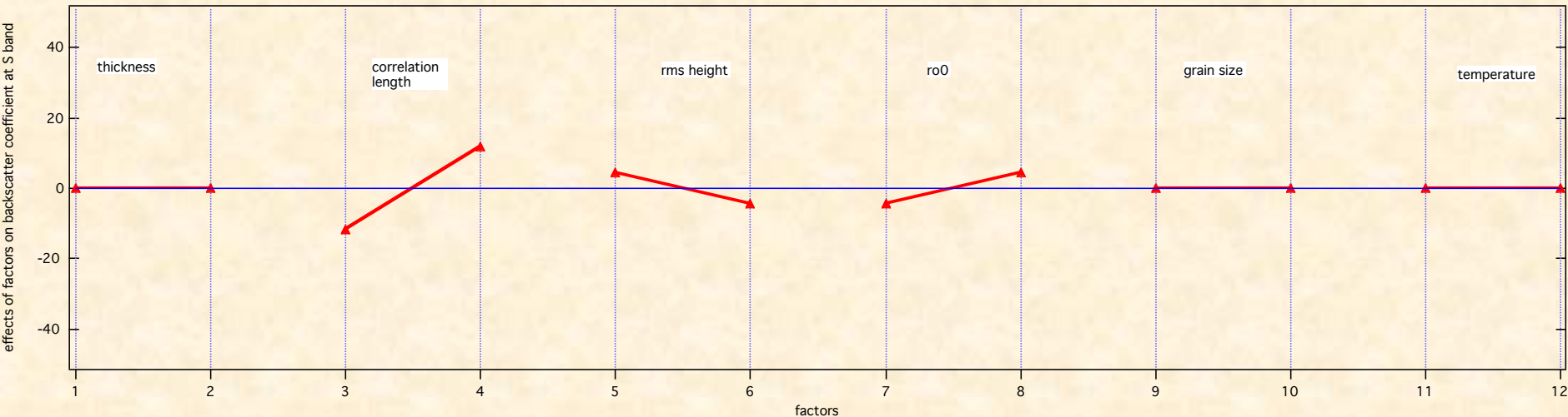
effects of factors on the backscattering coefficient S-Band (linear)
