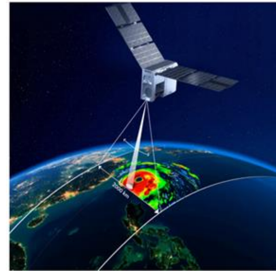
Tomorrow.io MWS sensor cross-track scan. Image from https://www.tomorrow.io/space/sounder/ .
